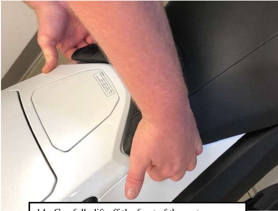
14. Carefully lift off the front of the seat
