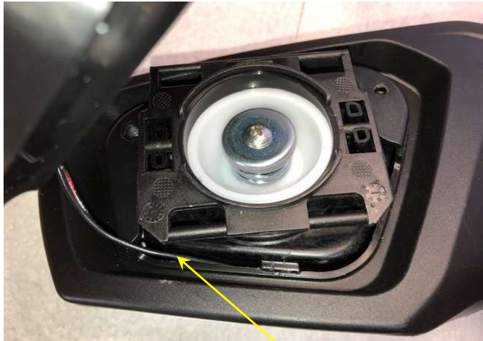
10. Ensure that the Signal mirror harness is not trapped before re-assembly of mirror housing. Correct positioning of wire is shown.
