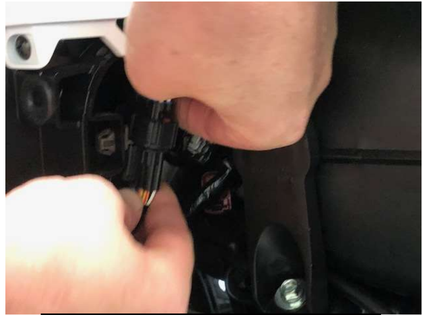
15. Unplug the seat heater connection
