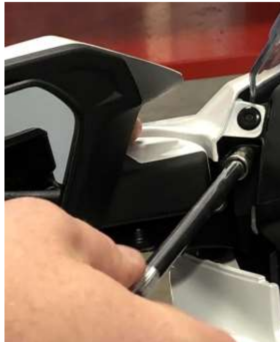
2. Remove the 2 mirror housing mounting screws.
