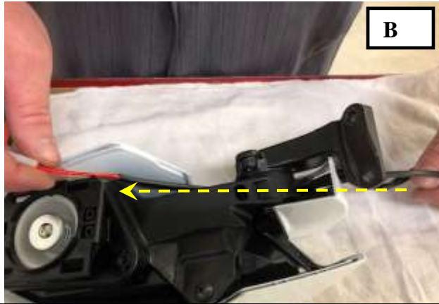
9. Route the Signal® mirror harness through the top side of the facia (photo A) and route the under-seat harness through the inside of the rear of the mirror shell (photo B)
