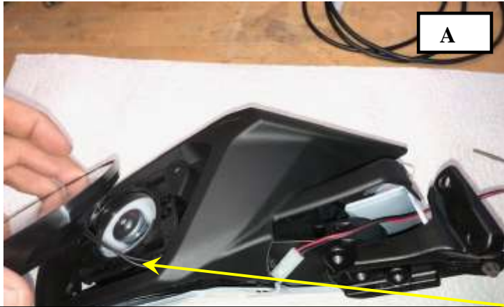
9. Route the Signal® mirror harness through the top side of the facia (photo A) and route the under-seat harness through the inside of the rear of the mirror shell (photo B)
