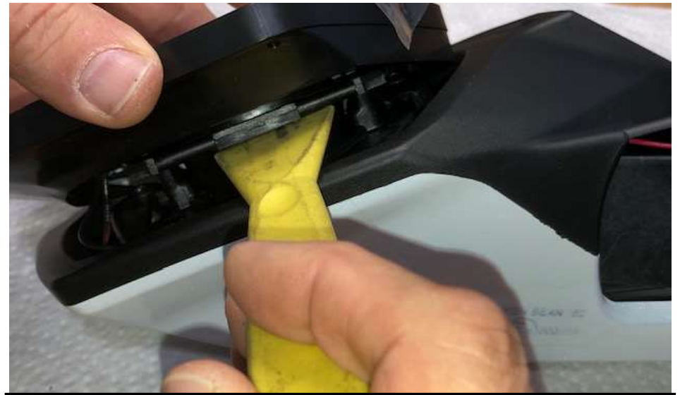
13. Insert the hinge hooks of the top of the mirror into the top openings of the housing actuator, then support the bottom of the actuator with a plastic pry tool and snap bottom of mirror into place.
