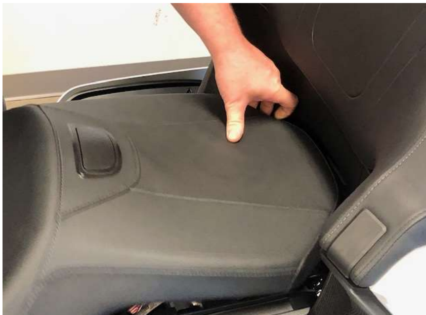
16. Wiggle the seat forward and remove seat.
