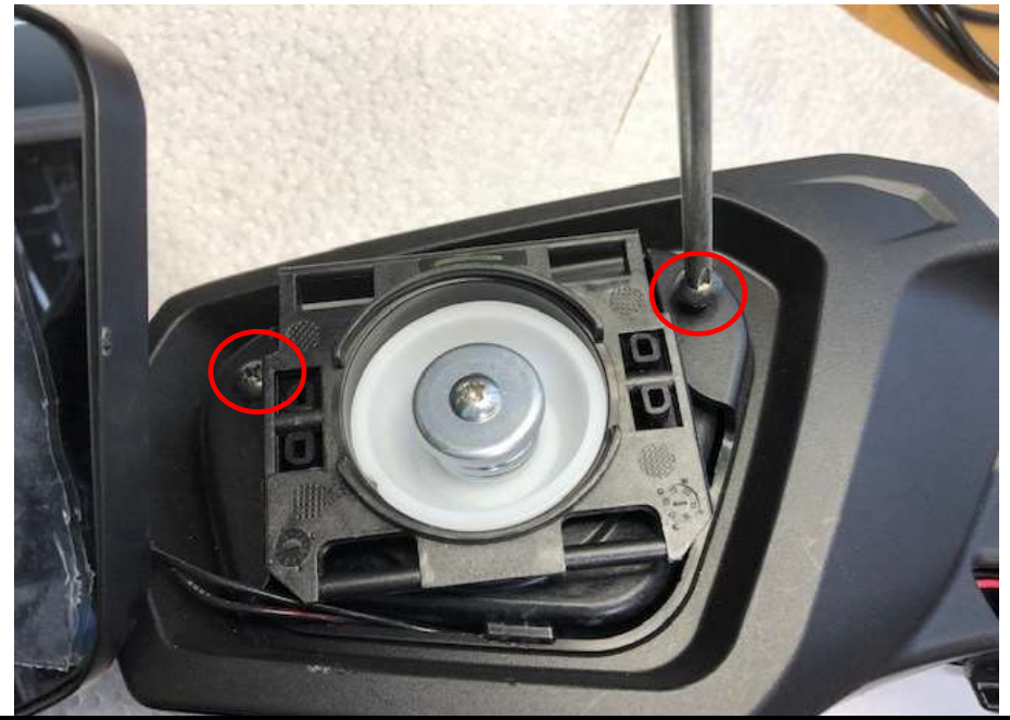
11. Snap the facia back into place on the mirror shell and replace the 2 screws.
