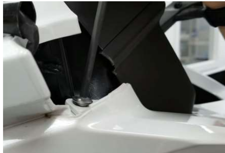
18. Remove one silver screw by mirror mounting area.
