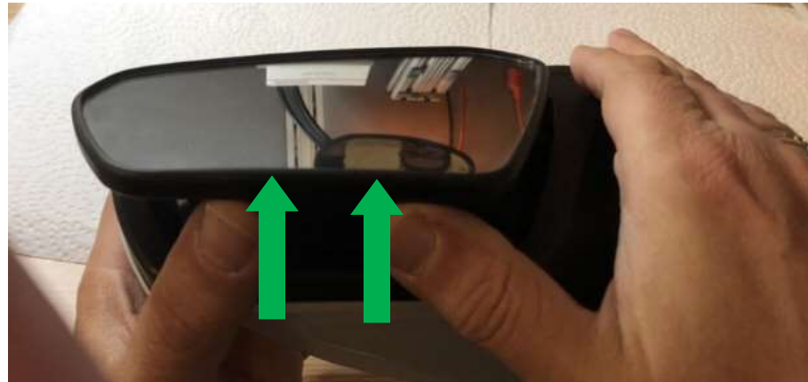
4. Place mirror housing on a clean, protected work surface. Unsnap bottom of mirror by prying firmly in an upward direction until the bottom of mirror unsnaps.
