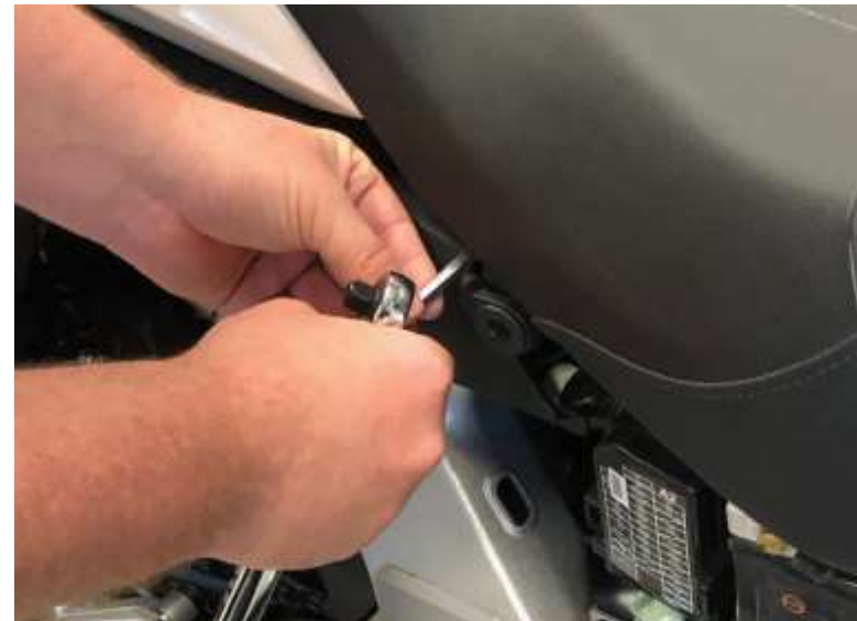
13. Remove (2) 6mm Allen screws from the front of the seat
