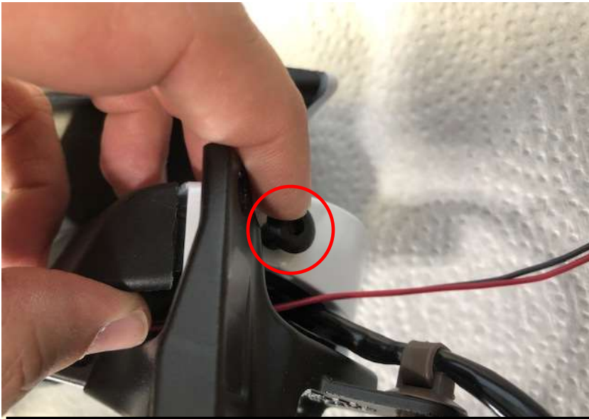
12. Replace the push pin at the inboard side of the housing.
